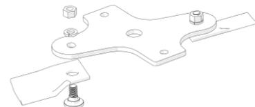
Pro-EzII Blade System installs on the same blade support bar as a fixed blade. This allows users to easily swap blade types as growing conditions or mowing requirements change.
