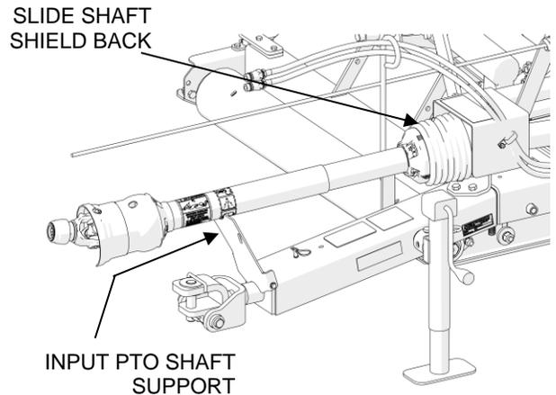
If the PTO shaft comes off during operation, it may cause personal injury and damage to the PTO shaft and tractor PTO. When checking, make sure the locking collar is locked, and that the shaft is not just jammed against the end of the tractor PTO shaft.
