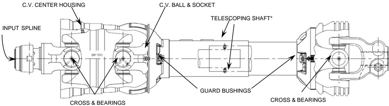
\* Inner & outer guards must be rotated to align holes for accessing the two telescoping shaft grease fittings.
