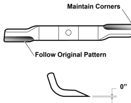
Figure 15– Grind Pattern
